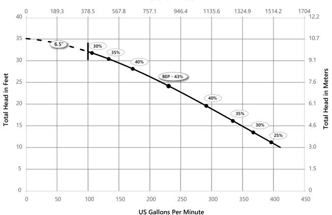
Stated efficiency values are Hydraulic efficiency. Wire-to-Water efficiency information is available upon request.
